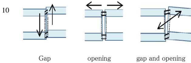
fig-6 Joint deformation overview
