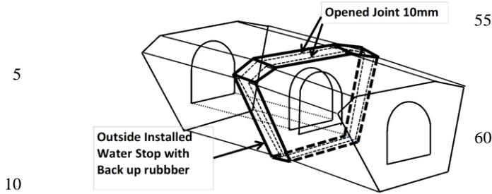
Fig. 11 Explanation of outside water stop structure
