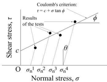
**Fig. 1** Schematic diagram of the in-situ rock shear tests.
