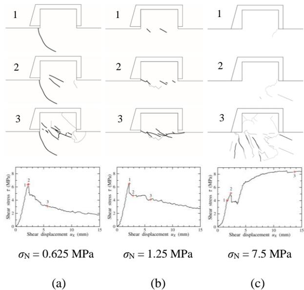
**Fig. 3** Crack sequences observed in three cases of the plaster model tests.
