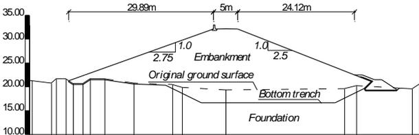
**Fig. 2 Cross section of dam (A-A)**
