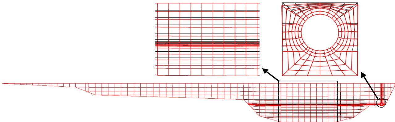
**Fig. 5 Deformation mesh of analysis (scale factor = 10)**
