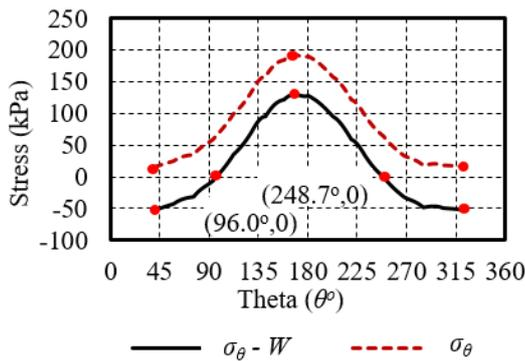
**Fig. 6 Graph of stress around pipe culvert versus theta angle ( $\theta^\circ$ )**
