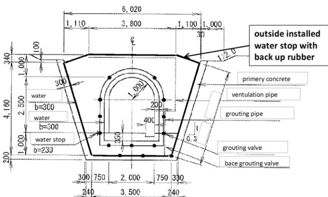
Fig.13 gallery Joint section with new type water stop
