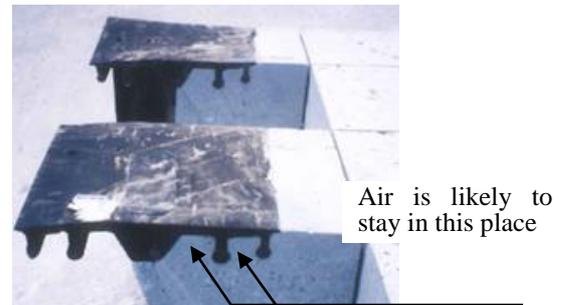
Photo 1 Casting test Specimen after cutting
