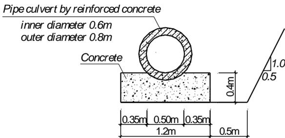
**Fig. 3 Cross section of culvert**
