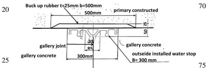
Fig. 12 Explanation of outside water stop detail
