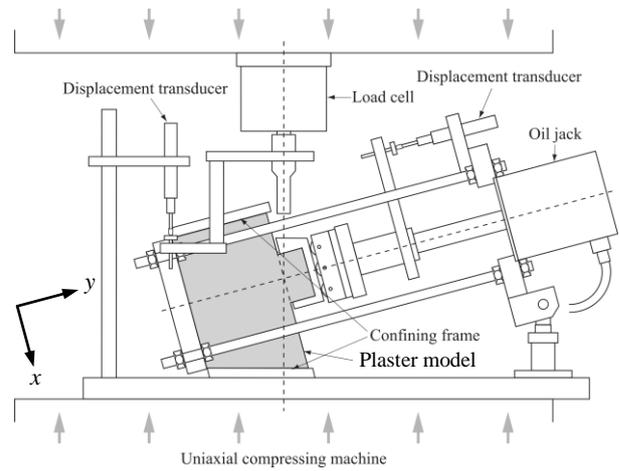
**Fig. 2** Brief description of the set-up of the model tests. The plaster model is shown in gray. The block part to be sheared is set as being inclined.
