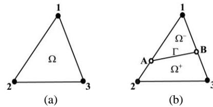
**Fig. 5** Finite elements to simulate cracks: (a) An ordinary triangular element; (b) An enhanced element including an interface  $\Gamma$  (Bolzon (2001)).
