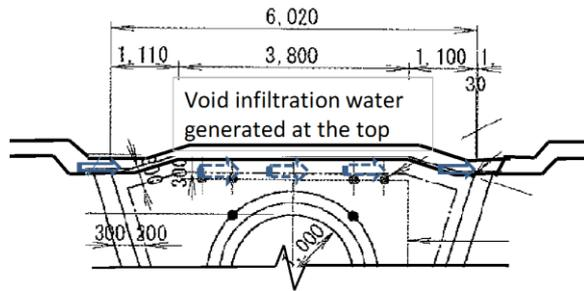
Fig.10 Opening formed between joints deformation on the top of the gallery joint
