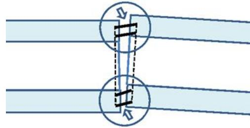
Fig. 9 Gap formed during joint deformation
