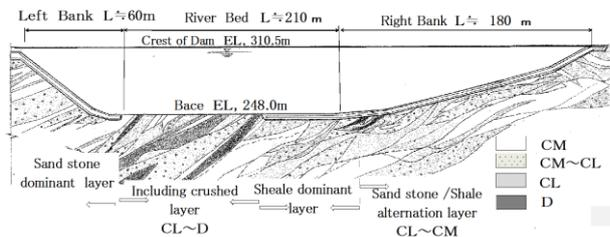
Fig-1 Rock classification longitudinal section
