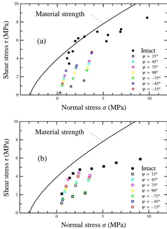
**Fig. 4** Shear strength: (a) Results of the model tests; (b) Results of the computation.
