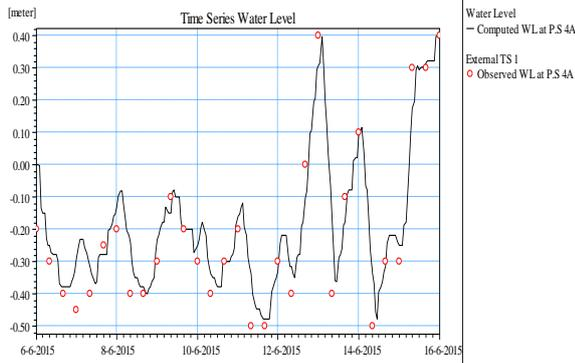
**Fig.5 Computed and observed water levels at the 4A pumping station (model verification)**
