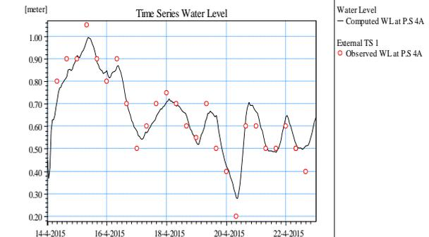
**Fig.4 Computed and observed water levels at the 4A pumping station (model calibration)**
