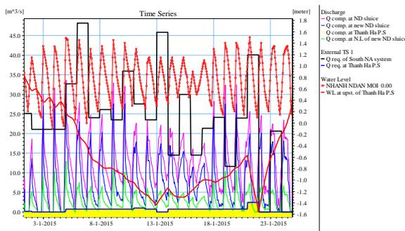
**Fig.7 Computed stage and discharge hydrograph and discharge requirement of the system and Thanh Ha pumping station (S8 – O3)**
