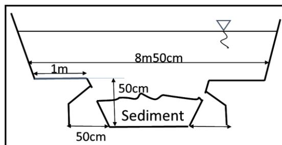
**Fig. 1 Cross-section of the Ooe drainage channel at a fish pool reach**
