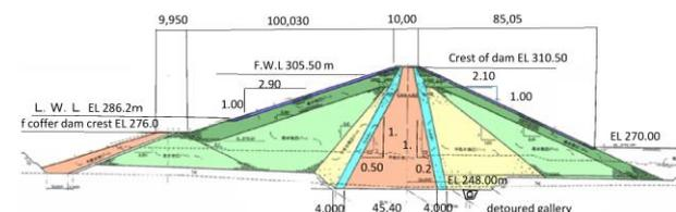
Fig. 5 Standard sectional of dam body
