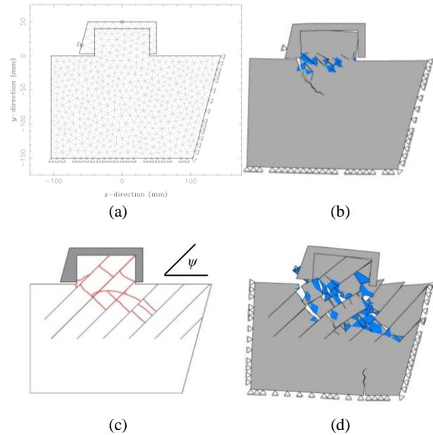
**Fig. 6** Results of the finite element analysis: (a) Discretization for the intact model. The normal force was imposed on the node enclosed with a circle. The inclined force was imposed on the node marked with a circle and a triangle, as the incremental displacement; (b) Results for the intact model,  $\sigma_N = 0.625$  MPa, whose results for the actual experiment are shown in **Fig. 3(b)**; (c) Cracks on the actual layered model,  $\psi = 45^\circ$ ; (d) Results for the same case as (c).
