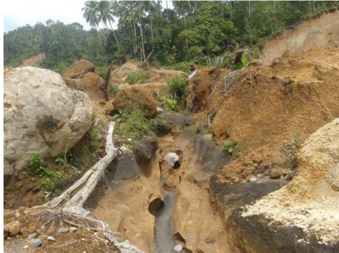
Figure 3 The soil that easy to erode by flow water because the soil is soft and weak from pumiceous tuff
