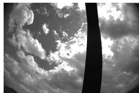
Fig. 4: Cloud image when solar irradiance changes suddenly. It's taken by sky camera. Black band in it is the shadow blade. (April 17, 2016. 13:07)
